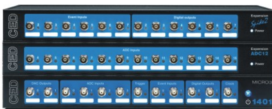
A selection of expansion units allows enhancement of the Micro3 to suit your application
