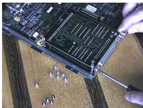
Remove the two connector plate screws
